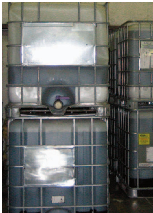
Rigid Nonmetallic Intermediate Bulk Containers (Picture courtesy of Chemical Specialties, Inc.)
